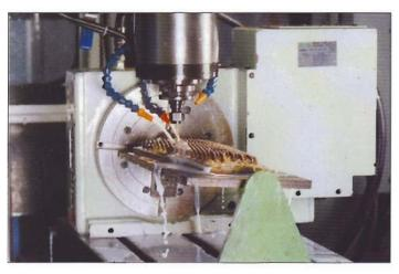
4 Axis CNC Machining center for Mfg. fillings of various applications. Ref. Chart.
