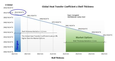
guarantees the minimum shell thickness variation throughout the whole length. The picture above shows the differences in drying performance that is acquired by the internal machining.
