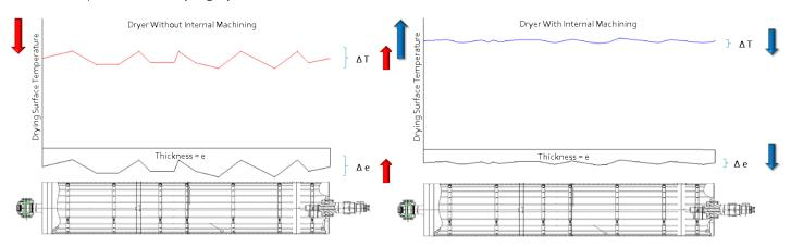
Besides the clear advantages when compared to cast iron ones, the dryers manufactured by Hergen feature a higher drying capacity even when compared with other steel dryers from the market, due the quite precise dimensional control, strict process monitoring and internal machining, which
