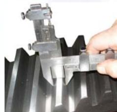
Gear wear and vibration are often symptomatic of other problems in the machine. Conditions like flooded dryers, bearings at or near failure, misaligned dryers or bearing housings, and overdrive & back drive are some of the problems that can be pinpointed during a **PTS** gear inspection.
