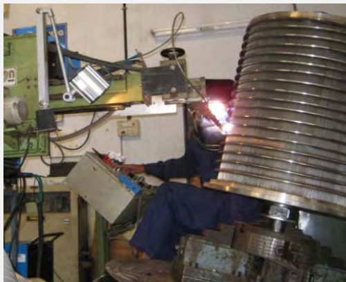
Wedge wire Welding
