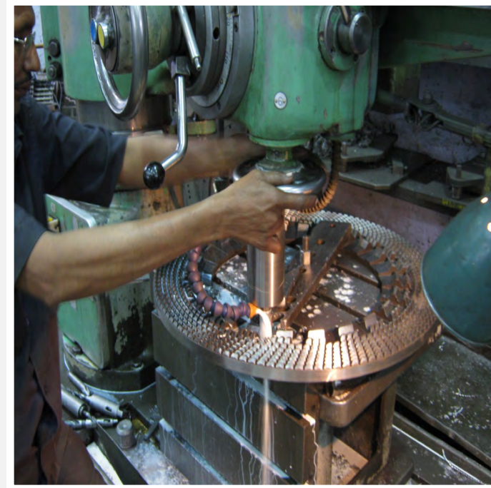
Drilling Holes / counters
