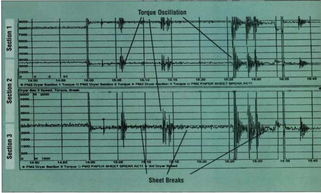
FIGURE 4: Based on torque measurements, this machine continues to experience cyclic torque oscillation spikes, which is still to be investigated.
