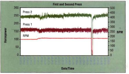
press drive motor was holding the first press roll back against the drive from the second press, which is transmitted through the shared fabric. Although the torque level on the first press in-drive shaft was not excessive, the overdrive can produce conditions detrimental to coupling life.
