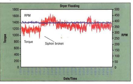
**FIGURE 6**: Torque measurements helped one mill determine that the torque increase coincided with a siphon break and subsequent flooding of one of the dryers.
