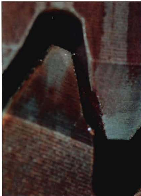
FIGURE 8: Excessive backlash can be caused by service-induced increases in the center distance between the mating gears.
