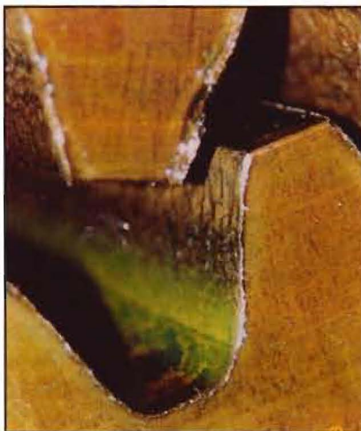
FIGURE 3. This photo shows misalignment caused by axial run-out.
