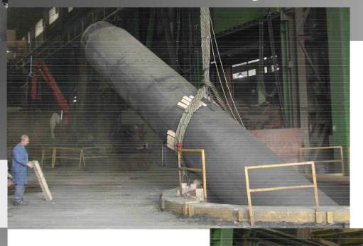
Roll is lifted from Casting Pit after one-to-two week cooling period
