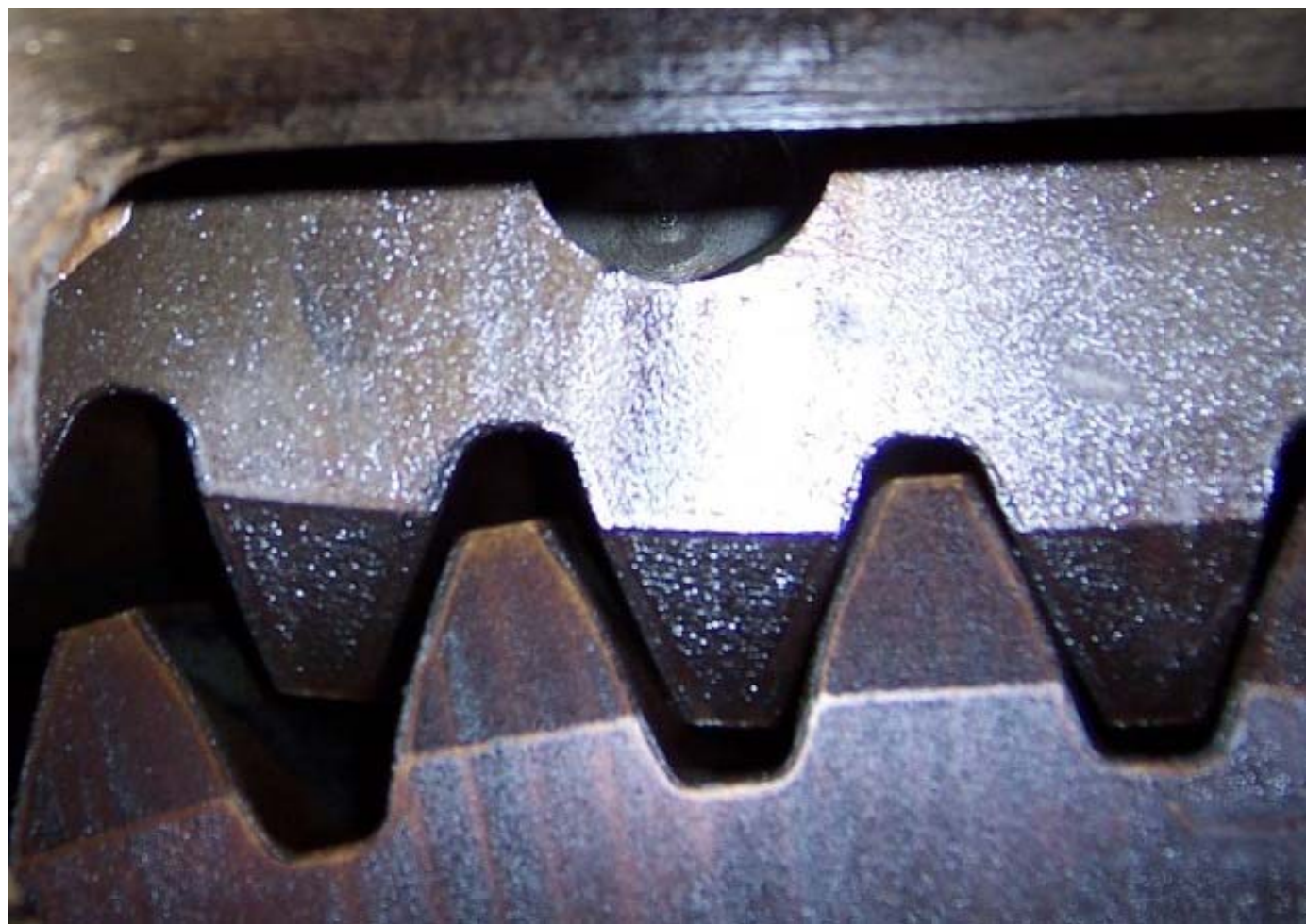
Older paper machine helical gear mesh with fair to good tooth profiles, and good backlash.
