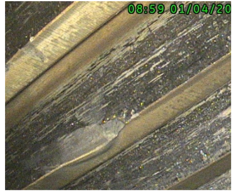
Video Scope Photo. Note cold flow of tooth edge; probably from contact with foreign matter.
